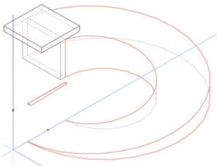
From the midpoint of the wall face that is parallel to the plaster line, draw a 6" [152.40mm] by 48" [1.219m] rectangle. Extrude to 4' [1.219m] and from the DS midpoint of this object draw a 4' [1.219m] by
