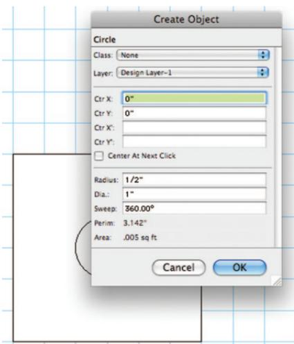
The circle has been added to the square. Let's make this a 3D object. Go to **Model>Extrude** (Command-E) and enter 3" [76.2mm] in the Extrusion field and click **OK**.
