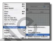
The Model Setup dialog box can be used to set up all the model layers for this project, but we will still need to add other layers to help us make this project. When you use this command on a new file, you get the first dialog box to set up the number of floors.
