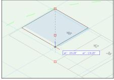
trim bottom Z should be 46", and the surface should be set to 42". (You'll have to do some simple subtraction, or you can let Vectorworks do the math by entering 48"-6" for the thickness of the surface.)
