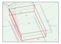
Extrude the Trim piece to 8" and set the bottom Z to 16". Repeat these steps to get the trim to the desired 2" height. Change the view, as needed, using the Flyover tool from the Basic Tool set. Toggle **Classes** and **Layers** on and off as needed.
