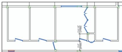
12. Press Shift + M for the **Move by Points** tool shortcut. In the Tool bar, enable **Move Mode**
