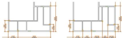
8. Press the X key, and then double-click each dimension and change the values to match the following figure (change the fixed point as necessary; see Notes below figure).
