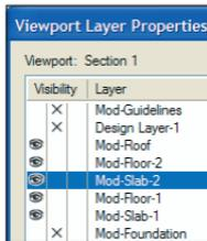
Sheet-Sections-1 sheet layer is activated (identified in the view bar as A4.1 [Sheet-Sections-1]), and the viewport is placed in the center of the sheet by default. Click in a blank area to clear the selection, and then select and delete the non-section viewport. Drag the section viewport into position, approximately where shown below.
