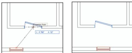
13. With the **Move by Points** tool still active, snap to the same midpoint on the window as the previous step, and then hold down the Ctrl key and snap to the insertion point of the master bathroom door's opening, as shown at left. The window is copied, and the copy is now centered with the master bathroom's opening, as shown at right (leave the copied window selected and the **Move by Points** tool active for the next step).
