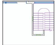
**Dimension Class Visibility** script to hide all dimensions. Press Ctrl + 6 to adjust the display, and then zoom in on the area shown above (notice the window sash width and depth changes from step 2). Right-click the floor to the left of the stairwell balustrade, and select Force Select. The Mod-Slab-2 layer is automatically activated.
