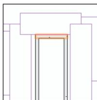
Next, you draw a rectangle, and then you use the **Wall End Cap** tool's **Add Mode** to join the rectangle to the pantry wall's core so that it extends to the exterior wall's core. You use the **Wall End Cap** tool because the **Wall Join** tool can't join these components in this particular configuration.
