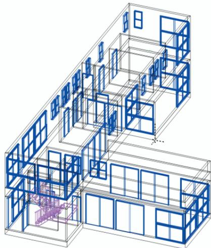
**Floor Plan-2** view. From the menu, select **View > Align Layer Views**. In the Scripts palette, double-click the **Toggle Dimension Class Visibility** script to hide all dimensions. Press Ctrl + 6 to adjust the display.
