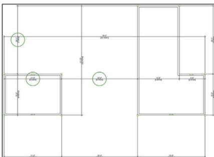
**18.** Right-click the text of the dimensions circled at left (one at a time), and select **Delete Dimension** from the context menu to remove them from the drawing. Drag the remaining dimensions (by dimension lines; not text) into place, approximately where shown at top below.
