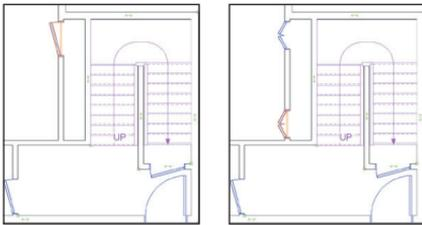
12. Use the Ctrl + drag method to copy the 3' [.914m]-wide foyer door to the left living room wall, approximately where shown below at left. In the Object Info palette, edit the new Door Width (7'0" [2.134m]) and Configuration
