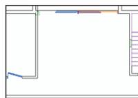
9. Repeat the **Create Similar Object** process to create a 7' [2.134m]-wide picture window from the first-floor plan and position it in the second floor's master bedroom wall, and then click outside the wall to orient it as shown at left. Use the Ctrl + drag method to copy the 7' [2.134m]-wide picture window eight times, approximately where shown at right (highlighted for clarity).
