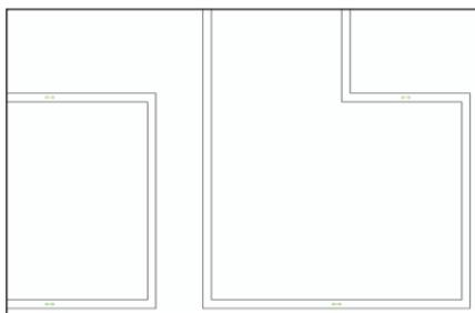
9. Press the X key and then drag one of the upper and one of the lower constrained walls to verify the constraints (both constrained walls move together), as shown at left. Press the X key twice to clear the current selection. From the View bar, click **Fit to Page Area**
