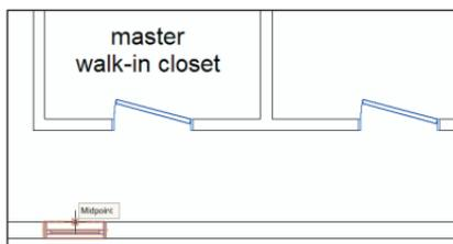
For the end point, click the insertion point of the master bedroom walk-in closet's door, as shown at left. The window stays in the wall and is now centered with the walk-in closet's door, as shown at right (leave the window selected for the next step).
