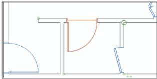
13. Use the Ctrl + drag method to copy the 3'-wide foyer door to the horizontal bathroom wall, approximately where shown above. In the Object Info palette:
