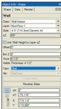
zoom in). Click the midpoint of the stair handrail's inside edge to resize the wall (and close the Snap Loupe), as shown at top right. In the Object Info palette, select **Start** from the **Caps** drop-down list, as shown at left.
