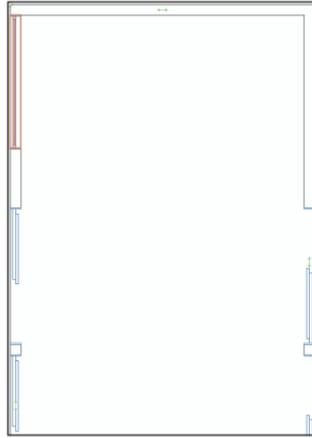
**16.** Press the X key, and then use the Shift + Ctrl + drag method (and the Ctrl + drag method) to copy the 7' [2.134m]-wide picture window seven times (highlighted for clarity) for a total of eight picture windows, as shown below (see Note).
