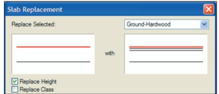
16. Repeat the Shift + select and replacement process for the second floor's floor slabs (select the **Mechanical-Duct Gap** slab style, and enable only the **Replace Height** option in the Slab Replacement dialog box). Clear the current selection so you can see the new slab style with additional components, as shown.
