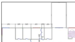
10. Repeat the **Create Similar Object** process to create a 2' [610mm]-wide window from the first-floor plan and position it in the second floor's master bedroom hallway wall, and then click outside the wall to orient it as shown (leave the window selected for the next three steps).
