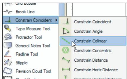
8. Click the midpoints of the wall segments in order, (shown below) to place colinear constraints between the midpoints and constrain the walls along their centerlines (notice the horizontal colinear constraint indicators  $\longleftrightarrow$ ), shown in the next figure. If either constraint fails, zoom in and try again.
