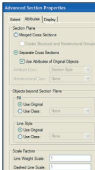
**of Objects Removed by Section** option, enable the **Show Wall and Slab Components** option, and then click **OK** twice. After several seconds, the viewport—with drawing label—is created, the
