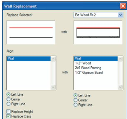
8. Repeat the **Select Connected Objects/** style replacement process for the three balustrade walls. Select **Ext-Wood-Balustrade** for the new style, and enable the **Replace Height** option in the Wall Replacement dialog box settings as shown, and then click **OK** to complete the replacement.
