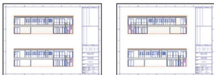
6. Shift + select the front elevation viewport. In the Object Info palette, verify that two Viewports are selected, and then click **Update** to hide the lines. Click in a blank area of the drawing to clear the selection and examine the elevations, as shown.
