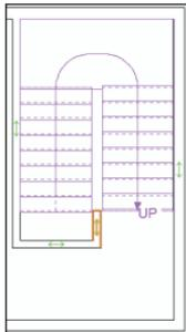
Click a blank area, and then select the stairwell wall. Click the top grip, hold down the Shift key, and then click the right front stair edge to resize the wall. Use the
