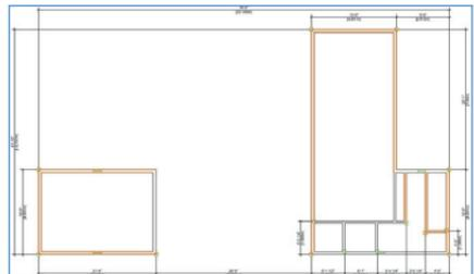
3. In the Object Info palette, verify that ten walls are selected, and then press Ctrl + C to copy them. In the Navigation palette, select the Saved Views tab, and then double-click the **Floor Plan-2** saved view to activate it (in the View bar, notice the Mod-Floor-2 layer is now active, as shown at right). From the menu, select **Edit > Paste** in Place to copy the walls to the same X and Y coordinates
