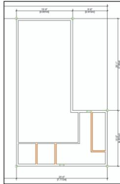
4. With the **Wall** tool still active, use the Shift key to draw a vertical wall segment—from top to bottom—connected with the vertical segment, approximately where shown.
