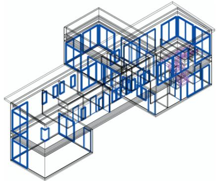
**Note:** The auto-boundary edge settings for the final slab styles' components automatically adjust wall component heights and/or slab component widths to create and maintain accurate junctions where walls meet floor and ceiling slab objects. You will see these junctions clearly after you complete the "Creating a section viewport" section (p. 72) and "Editing section viewport display properties" section (p. 74) in *Exercise 10*.
