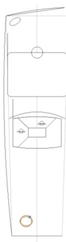
5. Use the Ctrl+drag method to copy the center function button (circle) to the center of the keypad oval, as shown at left. Click the circle's radius reshape handle, and then snap it to the oval's top center point to resize the circle's diameter to match the oval's height (.300 [7.62mm]), as shown
