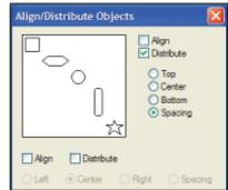
**27.** Press the X key twice to clear the selection, and then hold down the Shift key and select the keypad group and the locked vertical centerline. From the menu, select **Modify > Align > Align/Distribute**. In the Align/Distribute Objects dialog box, adjust settings, and then click **OK** to center the keypad group with the centerline. Press the X key twice to clear the selection, and examine the completed layout.
