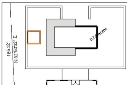
13. In the Resource Browser, double-click the **Ext-Siding-Framing** wall style to activate it. Press the X key and select the pool house rectangle. From the menu, select **Modify > Objects from Polyline**. In the Create Objects from Polyline dialog box, adjust settings as shown above (make sure the **Delete Source Poly** option is disabled), and then click **OK** to create the walls, as shown above at right. Leave the walls selected for the next step.
