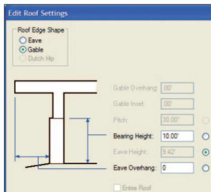
23. Select the garage roof's center left control point. In the Edit Roof Settings dialog box, select the **Gable** option, and then change the Eave Overhang to 0 (zero), as shown at top. Click **OK** to create the gable end and remove the overhang, as shown below.
