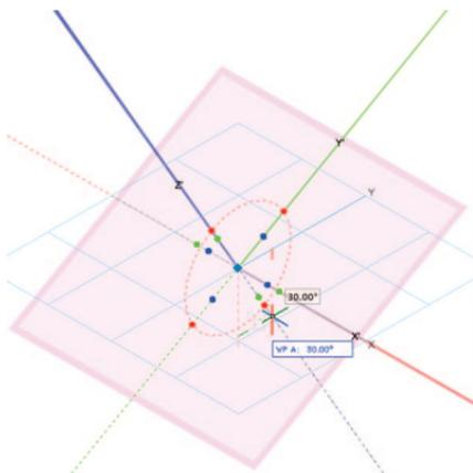
Select the Rectangle tool from the 2D tool palette and hover near the intersection of the axis. Note that you can click and draw on this new plane and that the cursor will “stick” to the 0-0 point at the intersection.
