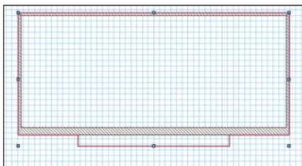
**Note:** Extruding objects with a positive value extrudes them up from the zero Z, and extruding with a negative value extrudes down from zero.
