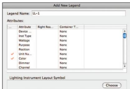
Click **OK**. Select **Edit Layout**, which will open the Edit Symbol window, defined by the colored border. From here you can select and drag the labels from the left column around the instrument. The Smart Cursor will help you align the data. You can also use the Align command. Text can be formatted from the Text menu. Click **Exit Symbol** when finished.
