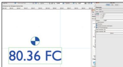
The Photometer tool in the Spotlight tool set measures the elevation and light at any given point on the stage. Draw Beam must be turned on for this tool to work. Simply select the tool and insert on the plot. As you turn Draw Beam on and off for different units or systems, you will have to refresh the Photometer Object.
