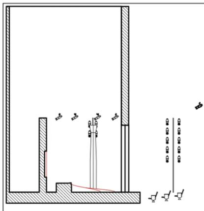
On the Model Layer you can rotate and position the booms so that they will appear correctly in sections and elevations using the 3D Selection tool in the Basic tool set or use **Modify>Rotate>Rotate 3D**.
