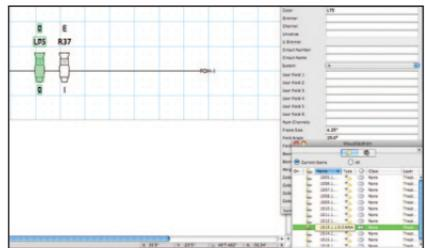
Also note that the instrument added now appears in the Visualization palette. Double-clicking on the instrument in the Visualization palette selects that unit on the plot.
