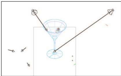
The Fill Light comes in lower and fills in places missed by the Key. Typically this is a softer light, so click and drag this light to be  $45^\circ$  from the Key Light. In the OIP, set the elevation to  $20^\circ$  and the brightness to 40% for this light, turn shadows off in the OIP.
