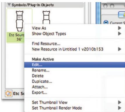
To Create a Hybrid symbol, edit the 3D component and copy the entire object. Exit the 3D and edit the 2D component and **Paste in Place** (Command-Option-V) the 3D element. With the 3D element still selected, go to **Modify>Convert>Convert to Polygons**, select the Hidden Line option. In the OIP set the Plane to Screen. Exit the Symbol.
